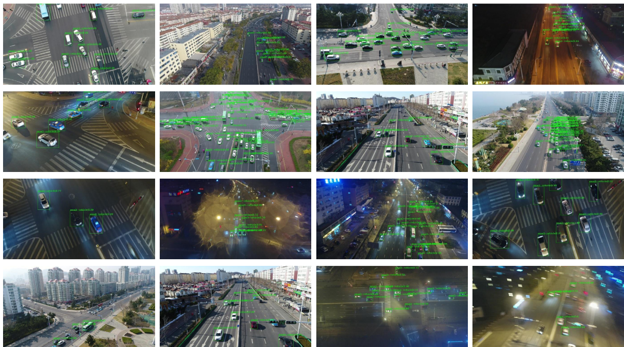
Fig. 6. The detection results in UAVDT dataset by the proposed multi-scale adversarial network. The detected vehicles are labeled with green rectangles and marked with categories and confidence scores. The last row shows selected images with wrongly detected or undetected vehicle objects. (For interpretation of the references to color in this figure legend, the reader is referred to the web version of this article.)
