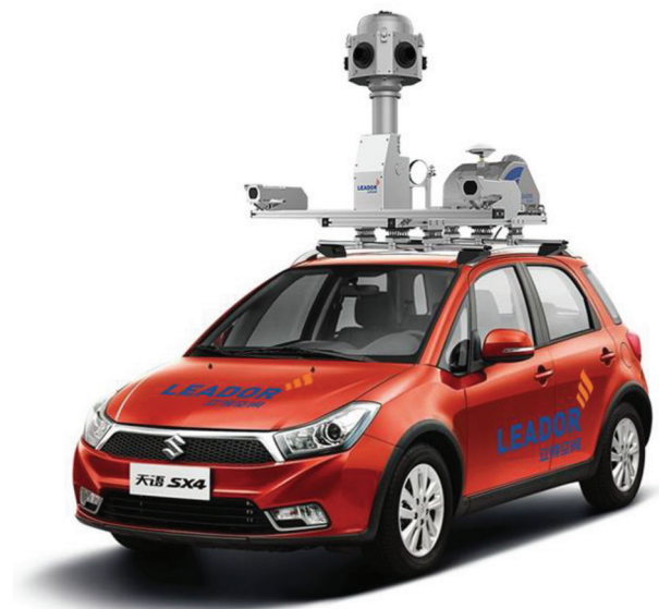
Figure 6. The mobile mapping vehicle system developed by Leader Spatial Information Technology Corporation.
