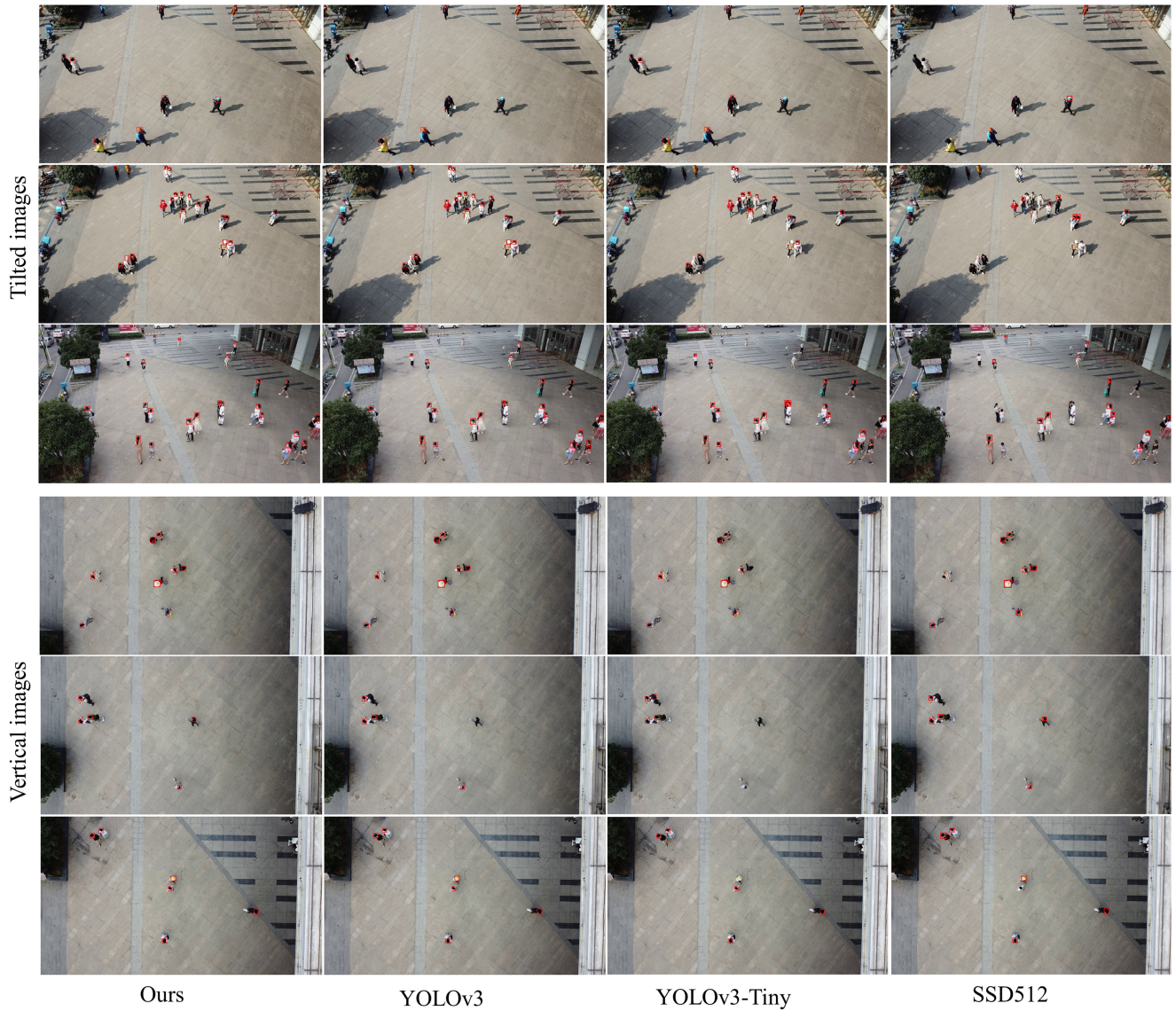
Fig. 14. The visualization detection results on UAV-Head dataset (including tilted images and vertical images).
