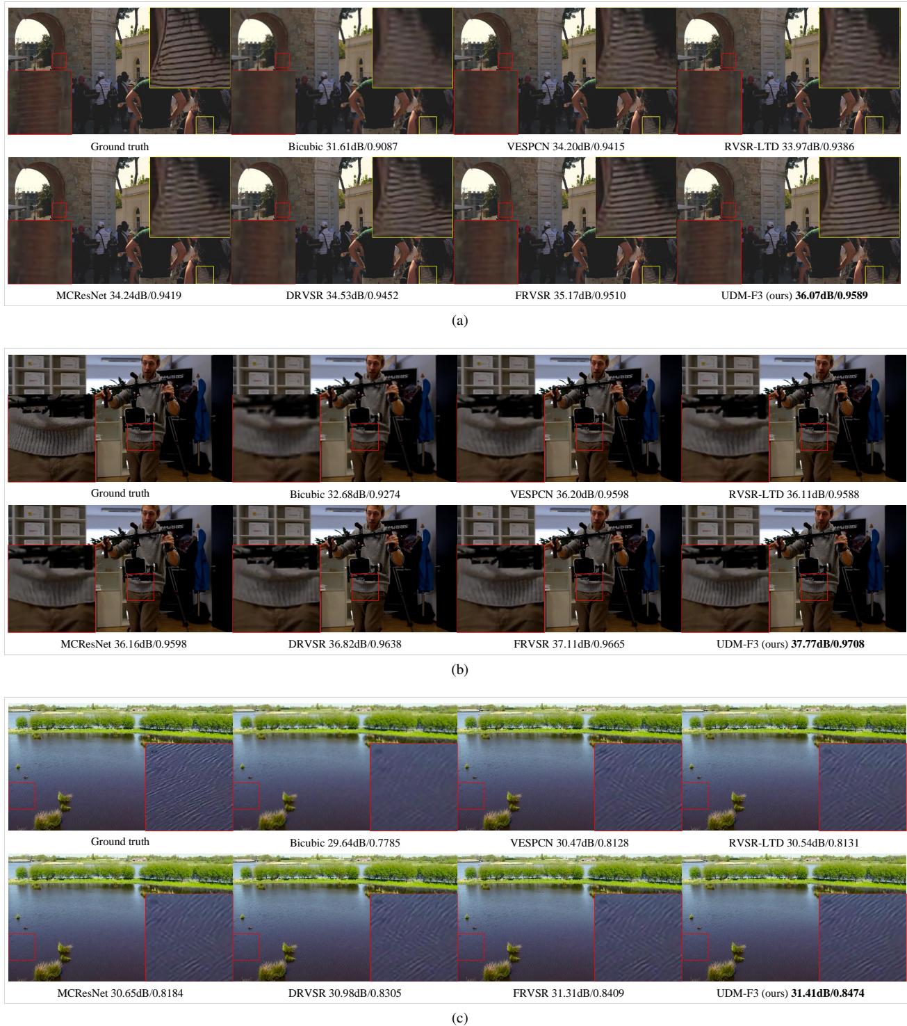
Fig. 7. Visual Results of different video SR methods. Upscaling factor is 4, and PSNR and SSIM are calculated by cutting off 8 pixels on each border. (a) This frame is from archpeople . (b) This frame is from photography . (c) This frame is from lake .
