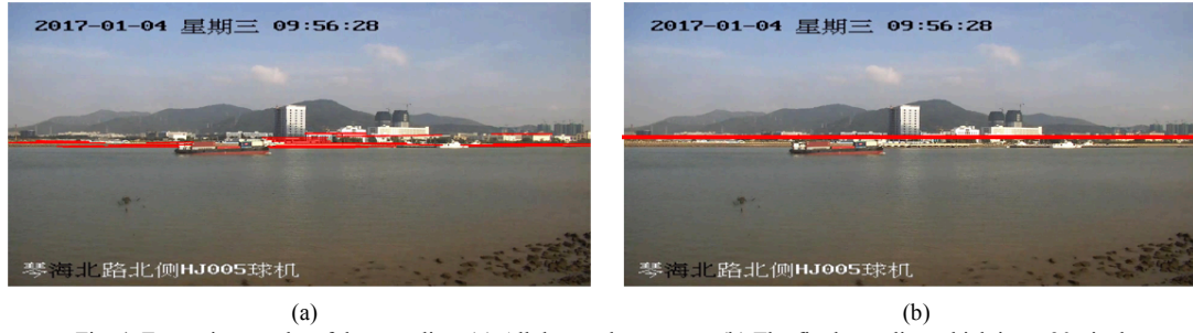
Fig. 4. Extraction results of the coastline. (a) All detected segments. (b) The final coastline which is up to 30 pixels.
