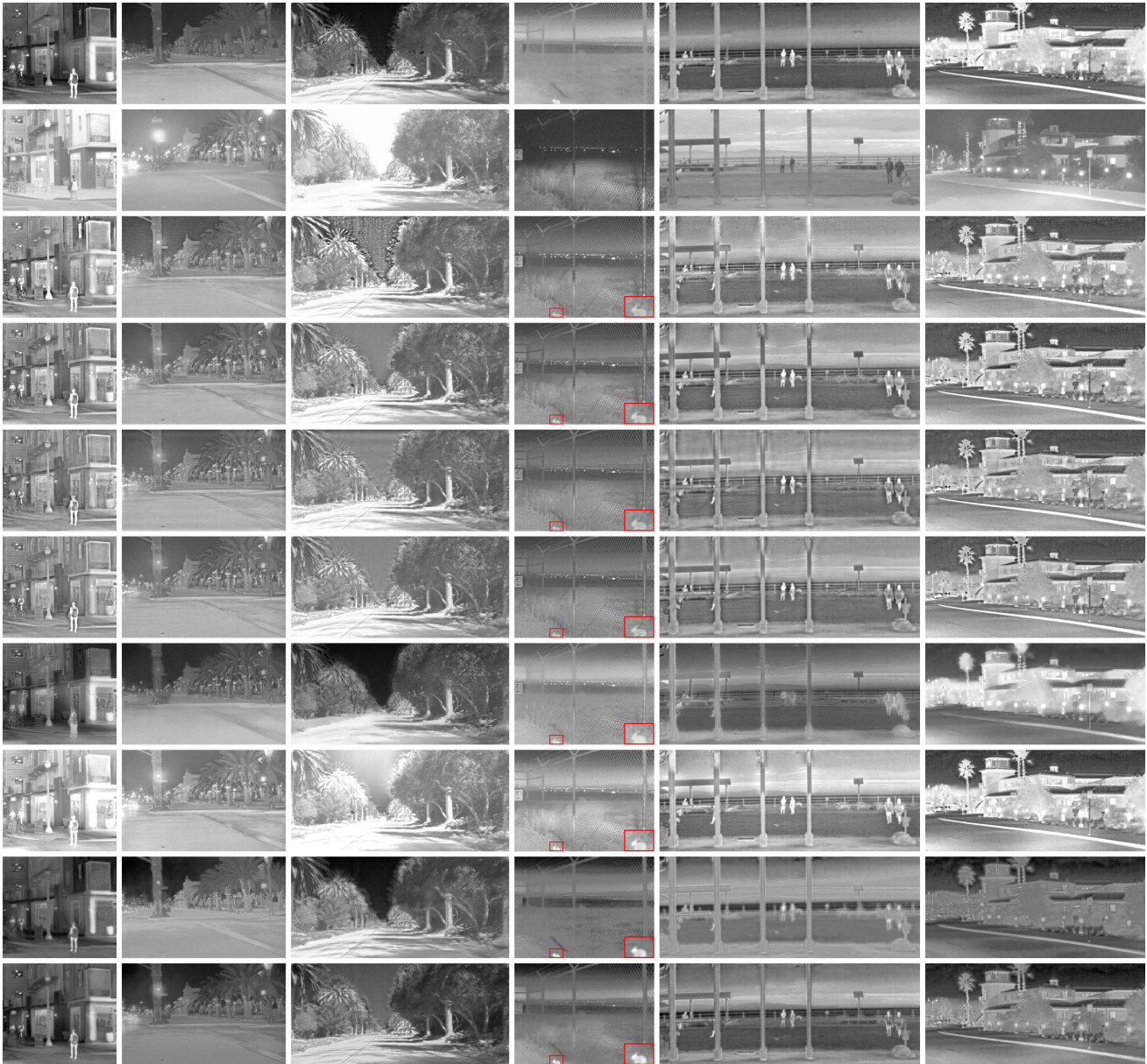
Fig. 9. Qualitative results on the RoadScene data set. From top to bottom: infrared images, visible images, fused results of LPP [44], LP [45], CVT [46], DTCWT [47], GTF [24], CNN [37], FusionGAN [16], and our GANMcC.
