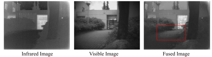
Fig. 14. Failure case. Unnatural shadow transitions appear in the fused image.
