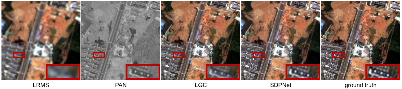
Fig. 1. Illustration of the pan-sharpening problem. From left to right: LRMS image, PAN image, pan-sharpened results of LGC [1] and our proposed SDPNet, and the ground truth (HRMS image).
